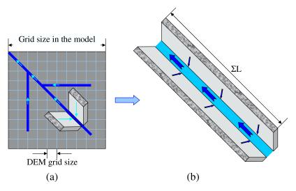
**Figure 2.** Simplification of streams in a model grid from (a) the DEM derived streams with a total length of  $\sum L$  to (b) one stream with a length of  $\sum L$ , which flows along the main flow direction of the model grid. Here a couple of geometrically symmetrical hillslopes are assumed to be located along one stream in both Figures 2a and 2b.
