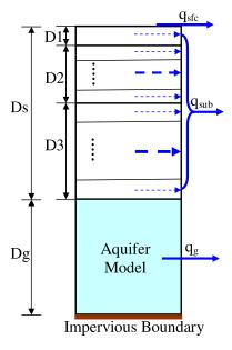
**Figure 3.** Soil model of the WEB-DHM. Two different soil subdivision schemes are used in describing the land surface and hydrological processes. The three-layer soil structure used in SiB2 is kept to represent the unsaturated zone in the calculation of land surface processes, and the unsaturated zone is divided into multiple sublayers when simulating vertical interlayer moisture exchanges and lateral subsurface runoff, as well as recharge from the groundwater aquifer.
