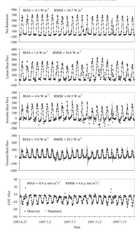
**Figure 6.** Observed and simulated energy balance components (unit: W m<sup>-2</sup>) and CO<sub>2</sub> flux (unit:  $\mu$  mol m<sup>-2</sup>s<sup>-1</sup>) at the NOAA flux site from 27 June to 19 July 1997.
