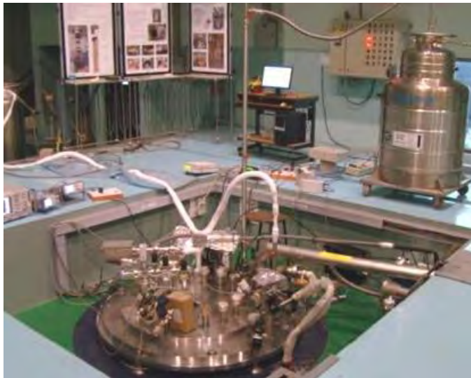
Single Cell LB 650 Cavity Developed at VECC/ IUAC and Tested at Fermi Lab
