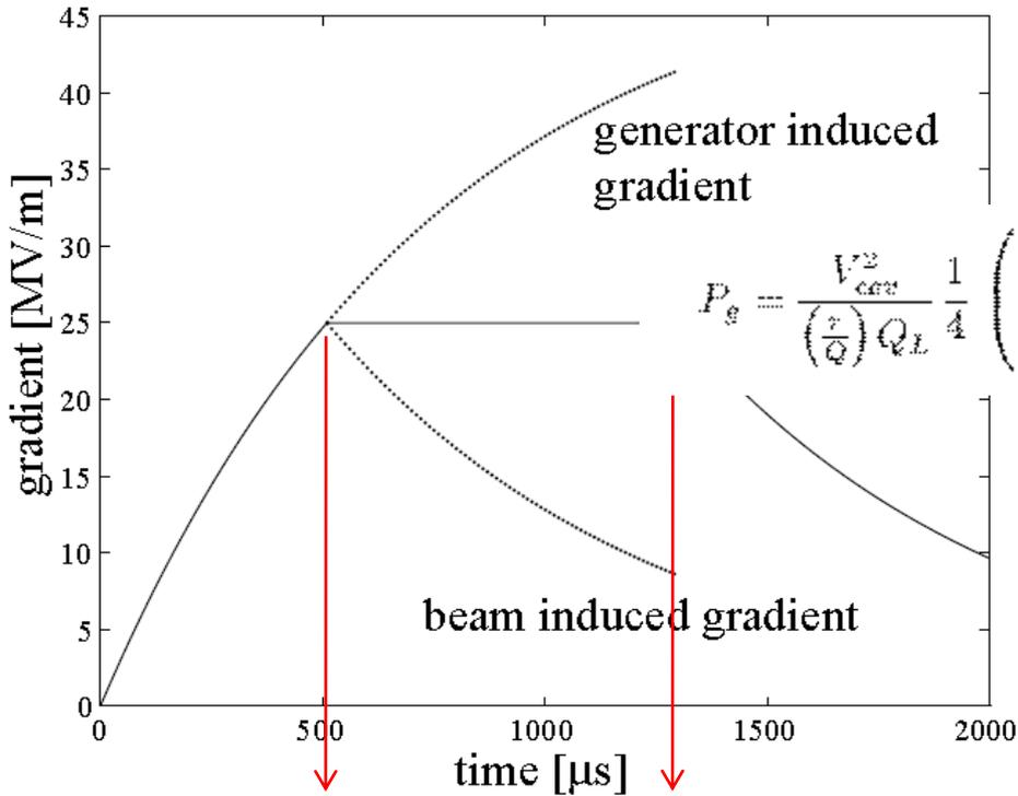
$$P_e = \frac{V_{\text{cav}}^2}{\left(\frac{r}{Q}\right) Q_L} \frac{1}{4} \left( \left[ 1 + \frac{\left(\frac{r}{Q}\right) Q_L I_{k0}}{V_{\text{cav}}} \cos \phi_k \right]^2 + \left[ \frac{\Delta f}{f_{1/2}} + \frac{\left(\frac{r}{Q}\right) Q_L I_{k0}}{V_{\text{cav}}} \sin \phi_k \right]^2 \right)$$
