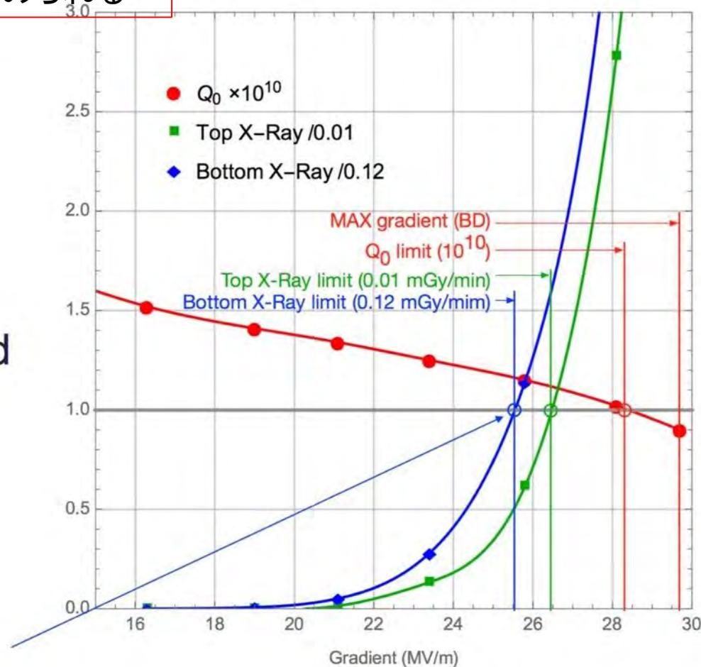
In this example, usable gradient is limited by FE (bottom X-ray) to ~25.5 MV/m
