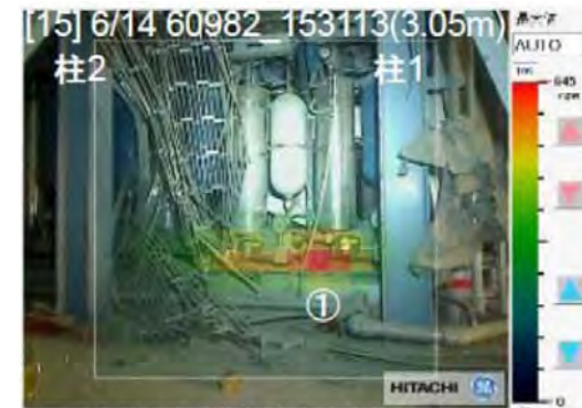
Radiation source survey( \gamma camera) results example (Unit 3 South side HCU)
