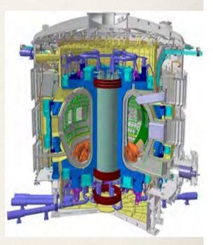
The incredibly complex ITER Tokamak will be nearly 30 metres tall, and weigh 23,000 tons. The ITER Tokamak is made up of an estimated one million parts.
