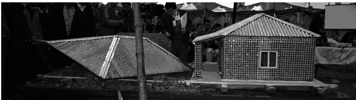
Totally collapse non-retrofitted model next to undamaged retrofitted one
