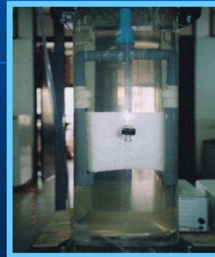
Solid liquid separation by microfiltration membrane
