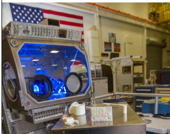
International Space Station's 3-D Printer
