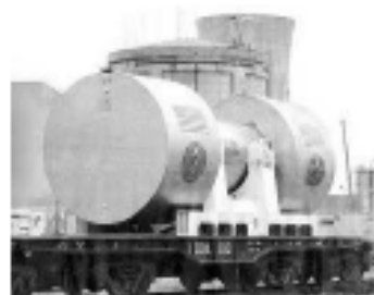
1986 to 1990 341 canisters of fuel & debris in 46 shipments by rail cask to the Idaho National Laboratory
