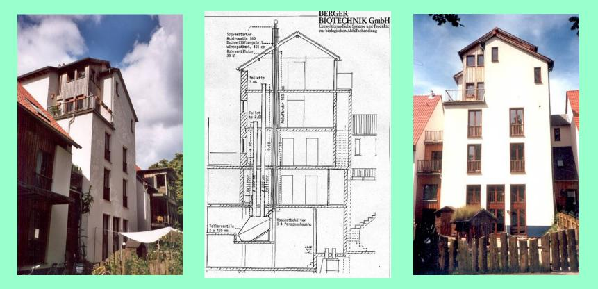
10 m down-pipe with 0,3 m diameter, 14 m exhaust air pipe, 0,15 m diameter, section USTB
