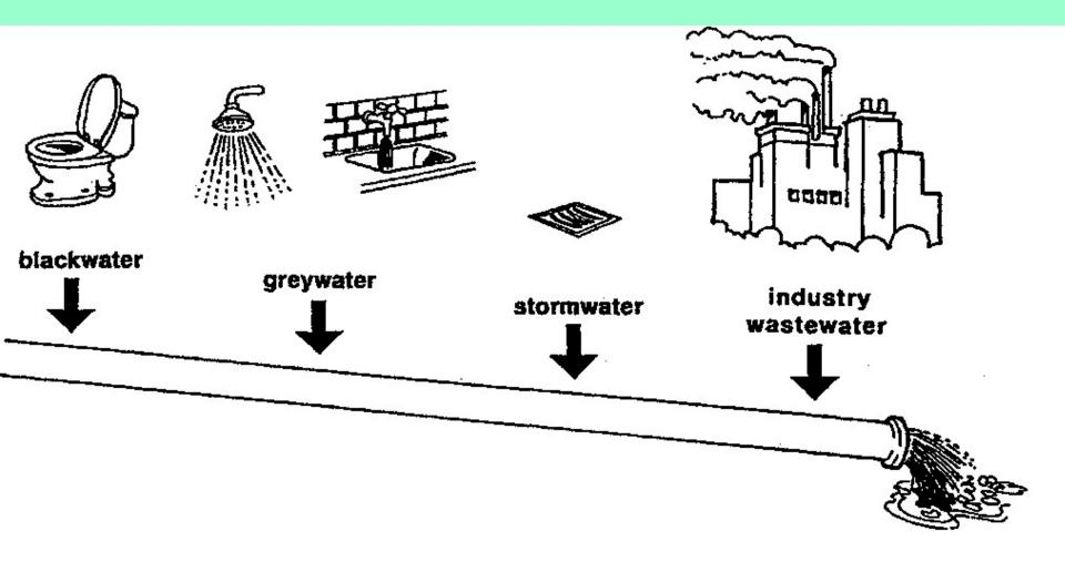
Figure 2: Conventional, "open" system (also called "end-of-pipe technology")
