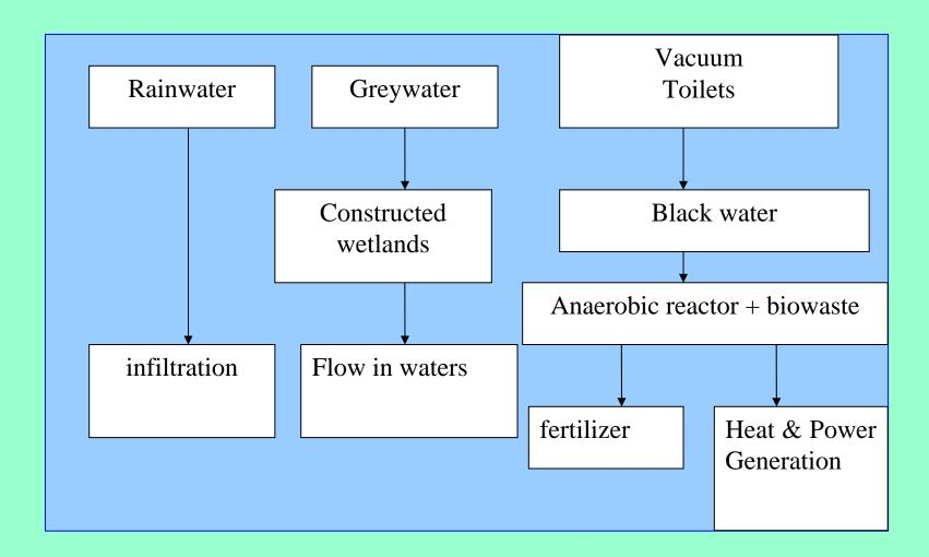
Figure 8: Schematic of wastewater treatment system with<br/>vacuum toiletUSTB
