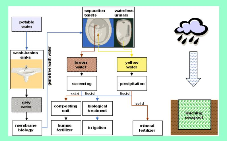
Figure 5: Schematic of wastewater treatment system with separation toilet (Company Huber, Germany)**USTB**
