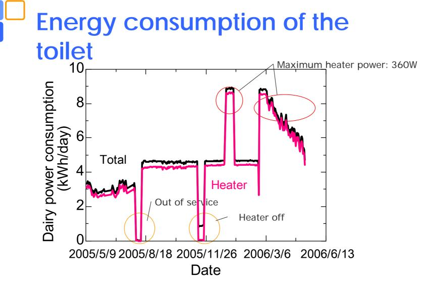
The electricity was consumed 3-9kWh/day (90-270kWh/month). Over 90% of it was used for heater.
