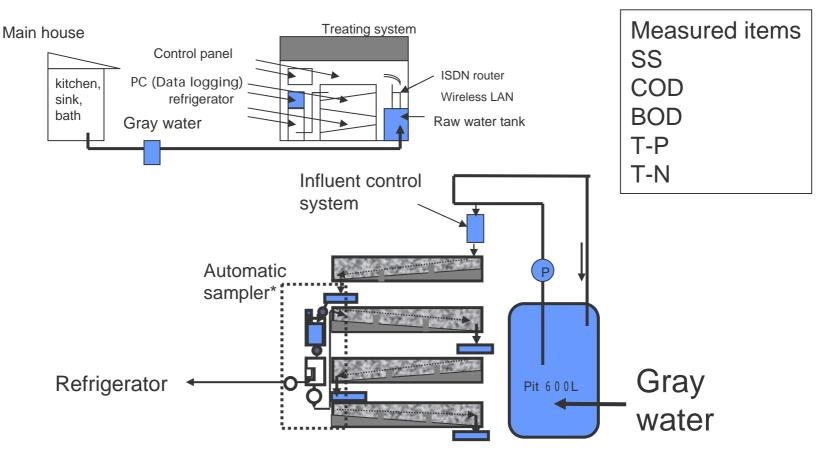
\* Automatic sampler: This device makes composites for all effluent.
