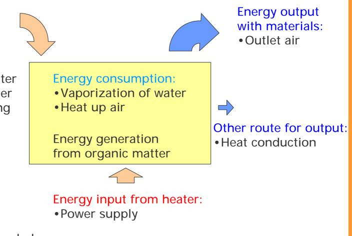
Energy balance: Accumulation = Input - Output + Heater + Reaction
