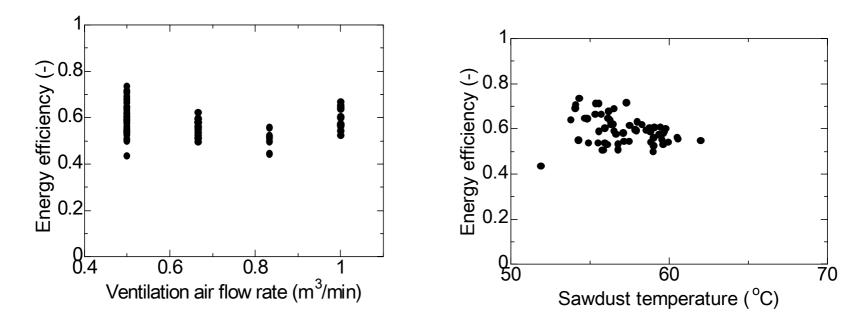
Slight effect of ventilation air flow rate and sawdust temperature
