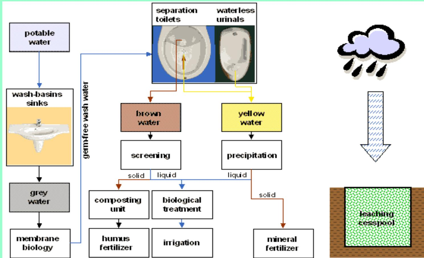
Figure 5: Schematic of wastewater treatment system with separation toilet (Company Huber, Germany)
