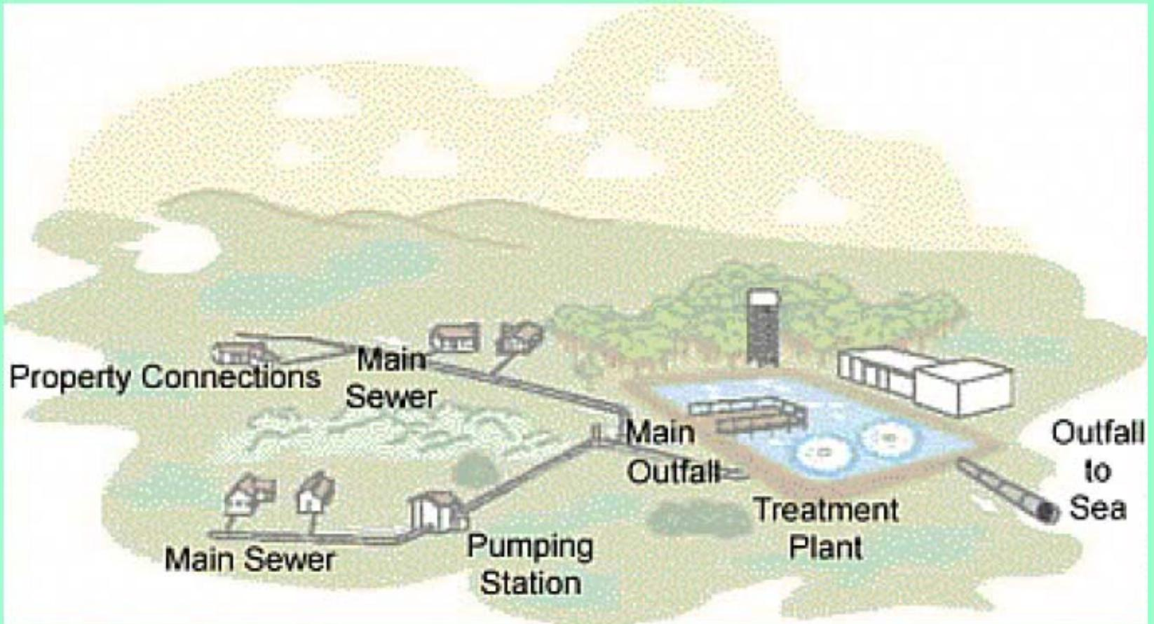
Figure 1: Conventional sewerage system
