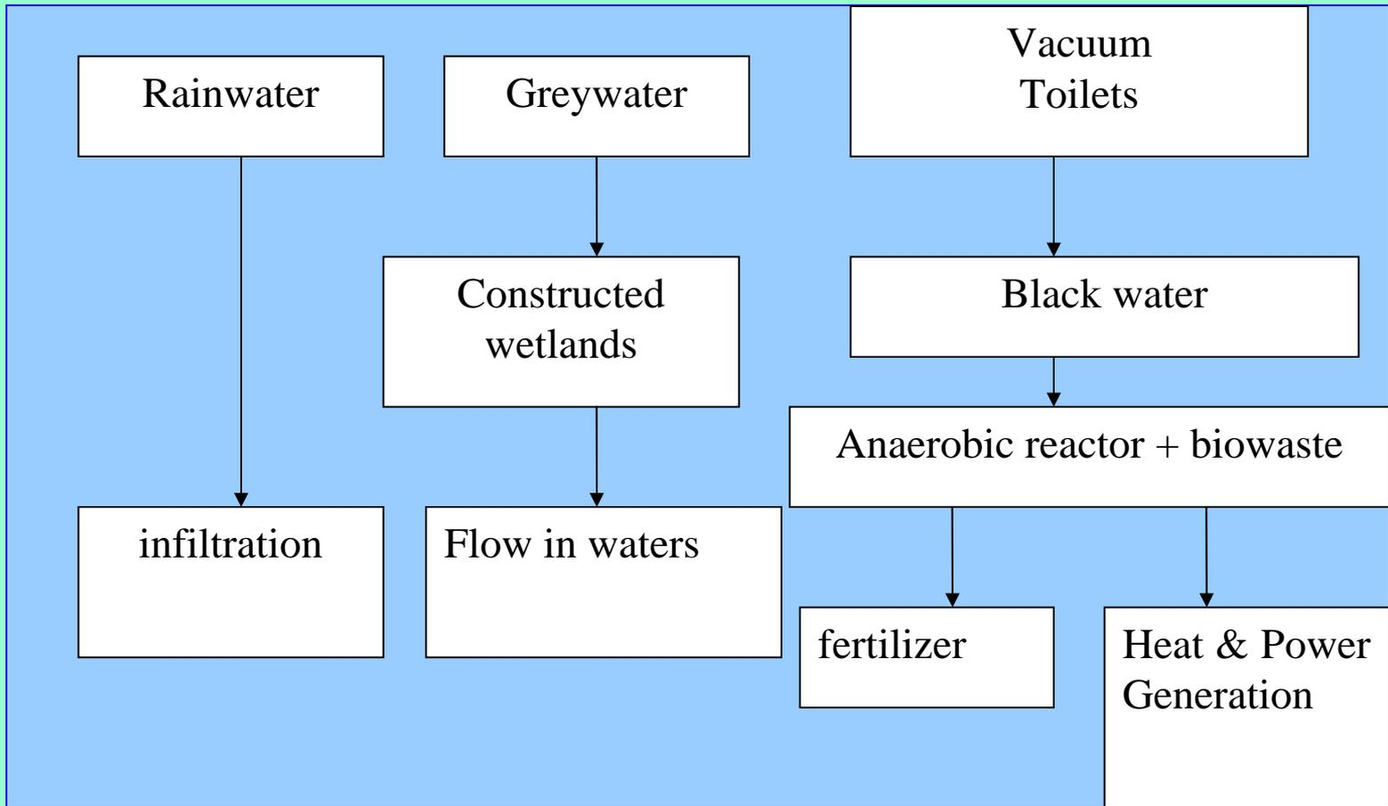
Figure 8: Schematic of wastewater treatment system with vacuum toilet
