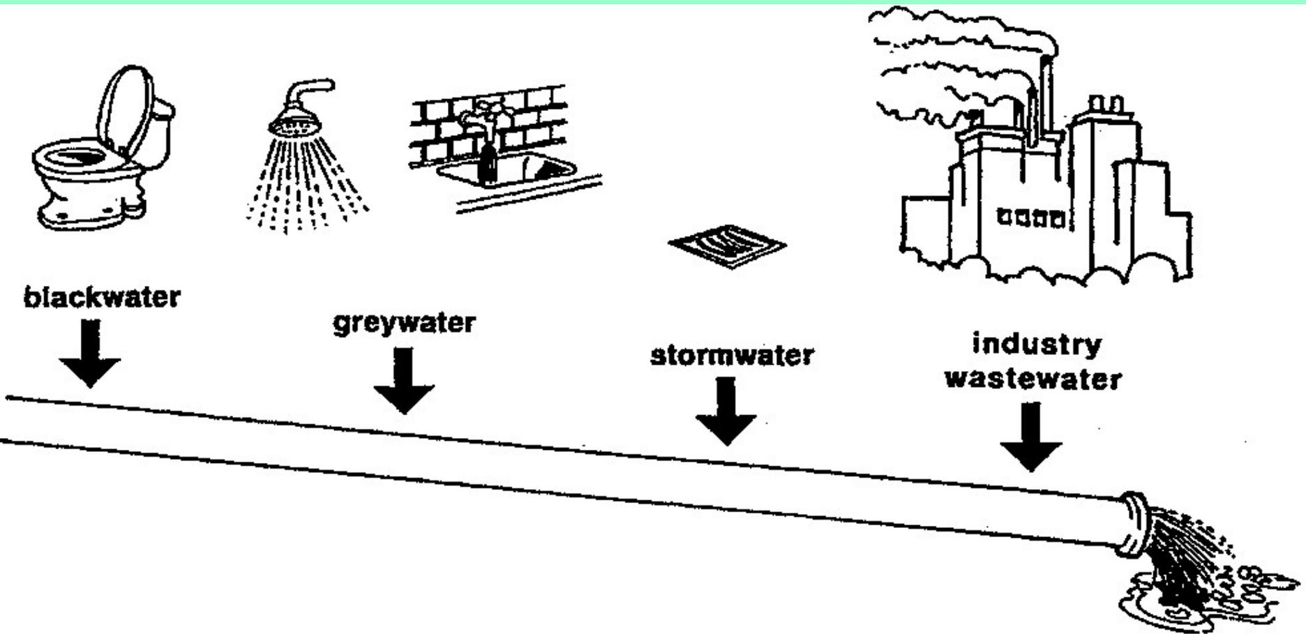
Figure 2: Conventional, “open” system (also called “end-of-pipe technology”)
