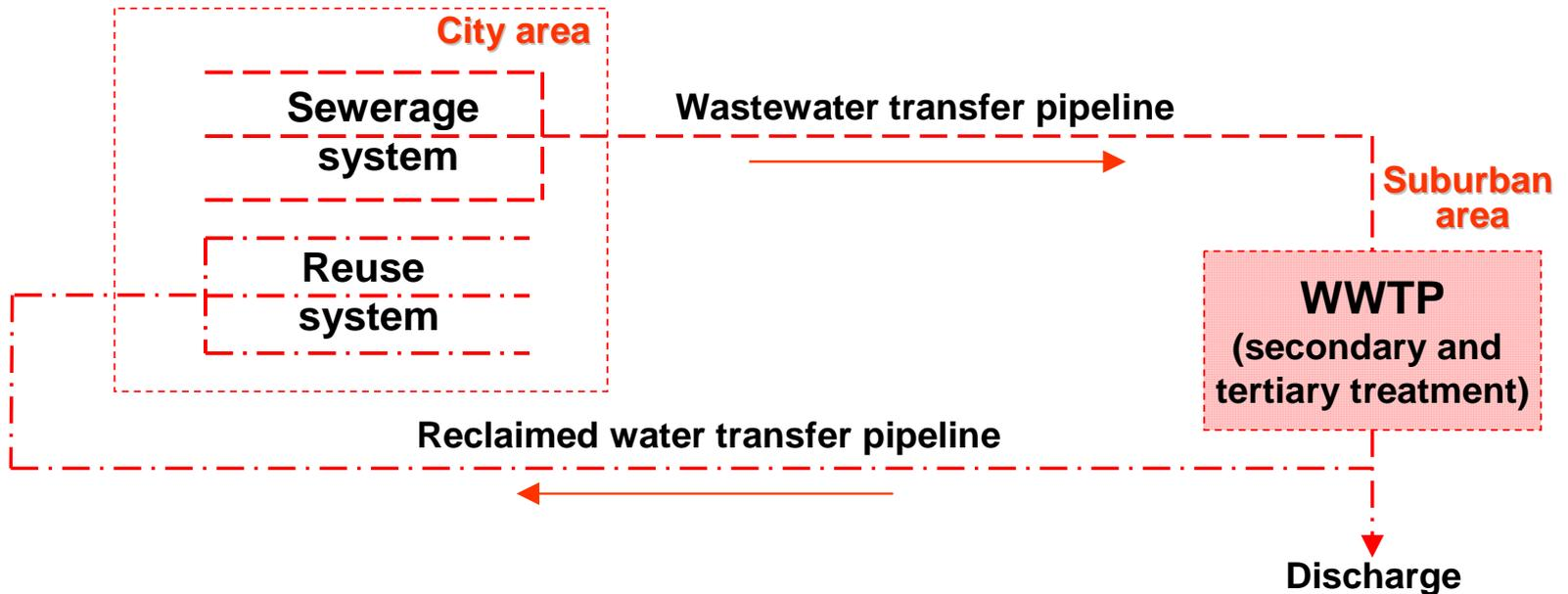
**In a modern city, the main purpose of the sewerage system is to carry away the wastes in a sanitary manner. Long distance transfer of the collected wastewater to the WWTP outside the city thus becomes a common practice. Another long distance transfer pipeline may have to be provided if water reclamation and reuse it to be practiced. This is also unwise because high construction cost and energy consumption are needed.**
