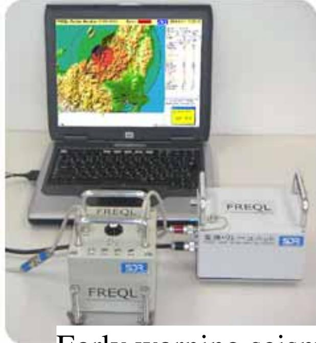
Early warning seismic intensity meter
