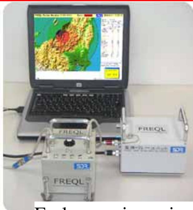
Early warning seismic intensity meter
