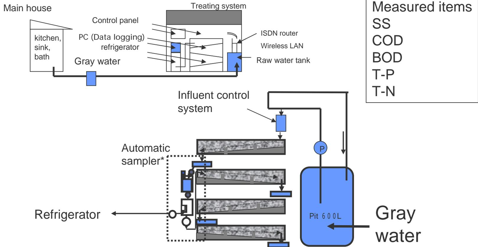
\* Automatic sampler: This device makes composites for all effluent.
