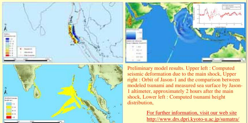
Preliminary model results. Upper left : Computed seismic deformation due to the main shock, Upper right : Orbit of Jason-1 and the comparison between modeled tsunami and measured sea surface by Jason-1 altimeter, approximately 2 hours after the main shock, Lower left : Computed tsunami height distribution,
