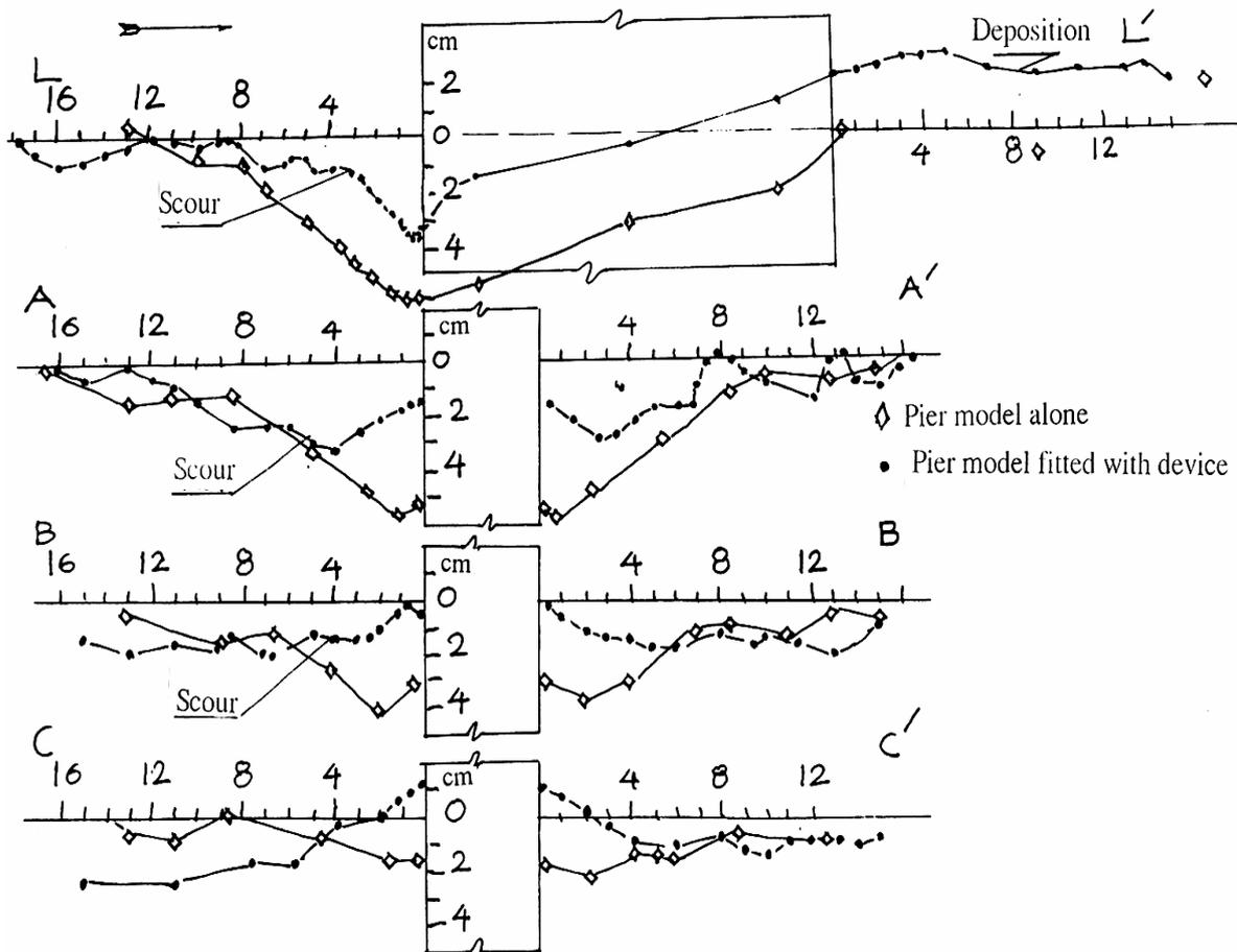
Fig.9a. The change of sense of scour depth and reduction scour depth around pier model fitted with device.
