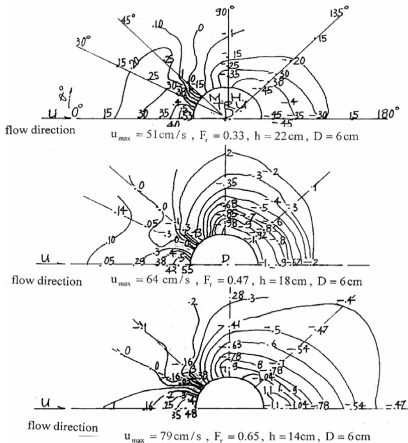
Fig.4. Pressure contours on plate before scour
