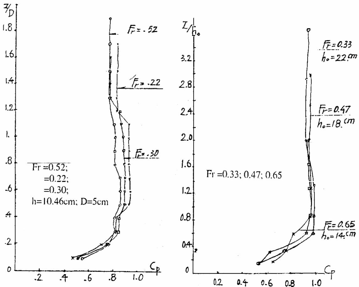
Fig. 5 . Pressure coefficient variation along the line of symmetry or  $\theta = 0^\circ$  on pier model surface.
