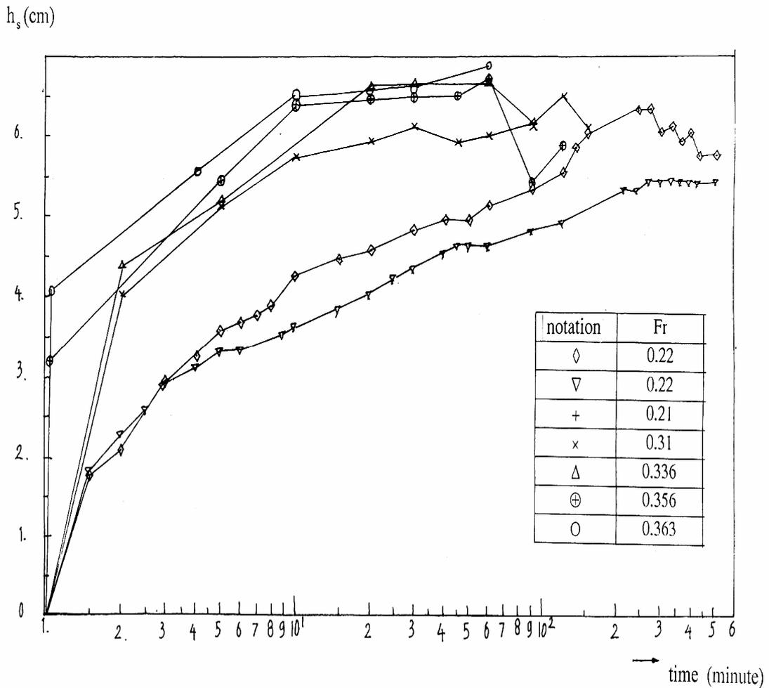
*Fig.6a. Variation of scour depth versus time for pier model alone
