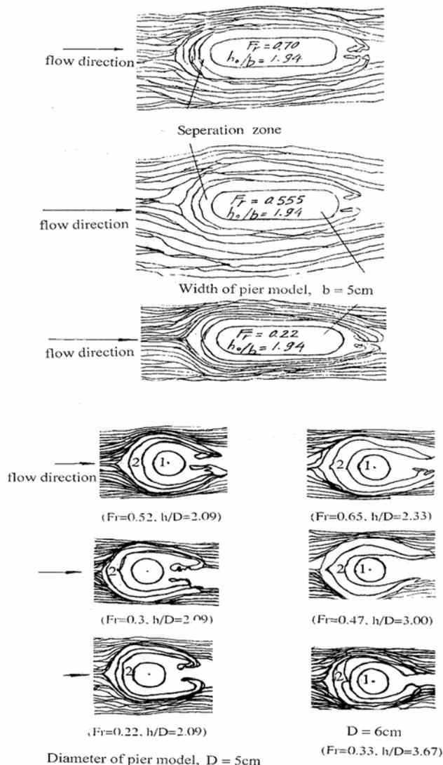
Fig.1a. Paint impression of flow pattern on the plate for pier model alone.
