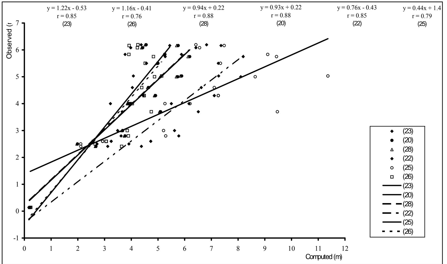
Fig.11. Comparison between Eq. (20), (22), (23), (25), (26) & (28) for live bed scour
