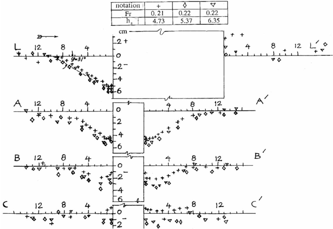
Fig.6b. Scour hole shape and depth around the round nosed pier model for width  $b = 5\text{ cm}$ ,  $Fr = 0.21 ; 0.22$ .
