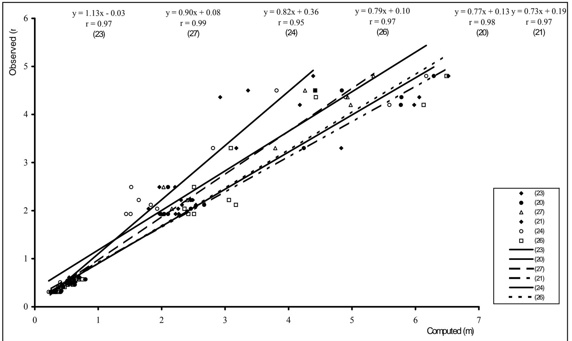
Fig.10. Comparison between Eq. (20), (21), (23), (24), (26) & (27) for clear-water scour
