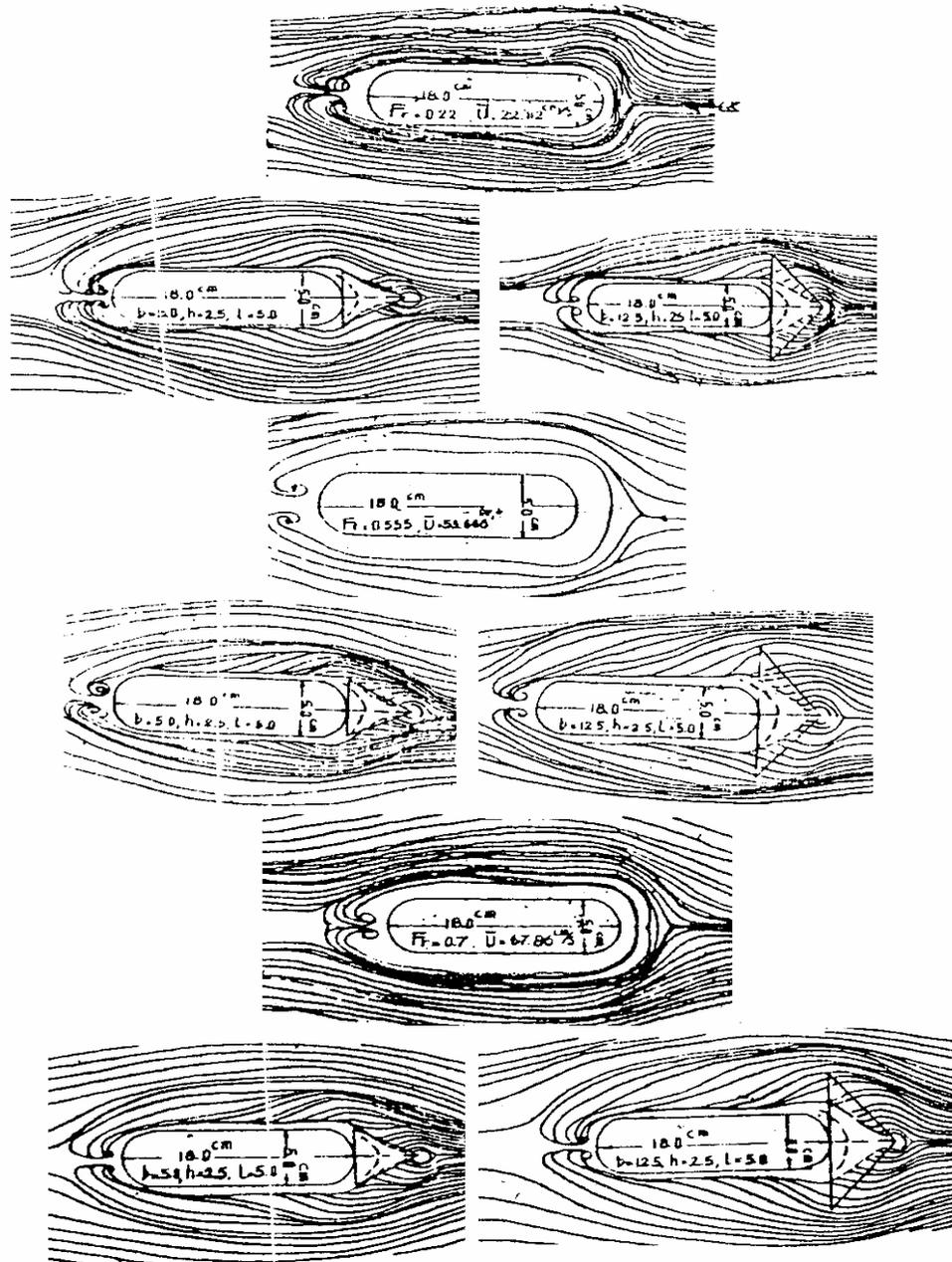
Fig.1b. *Paint impression of flow pattern on the plate for pier model alone and fitted with device model. for  $Fr = 0.22; 0.55; 0.7$*
