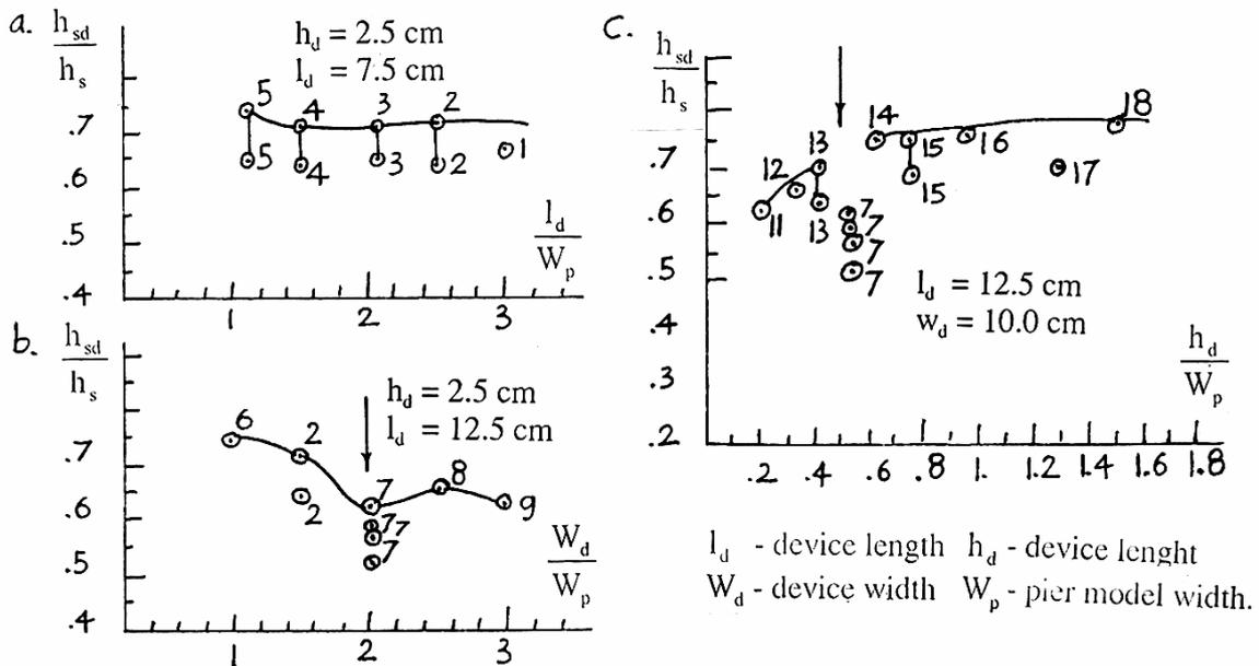
Fig.8. The most effective dimensions of delta-wing-like passive device based on effective hydraulic reason.
