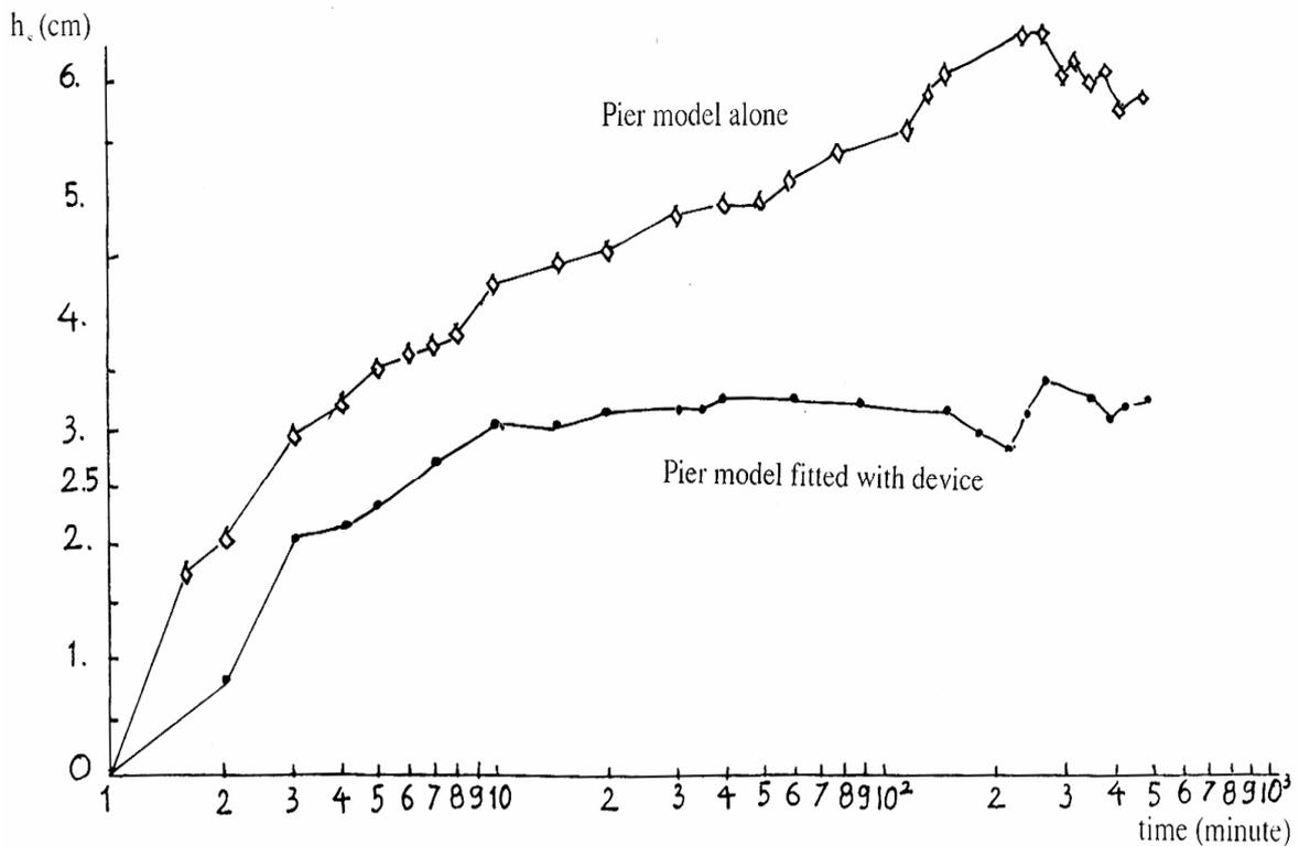
Fig.9b. Comparison of scour depth versus time for pier model alone & fitted with device
