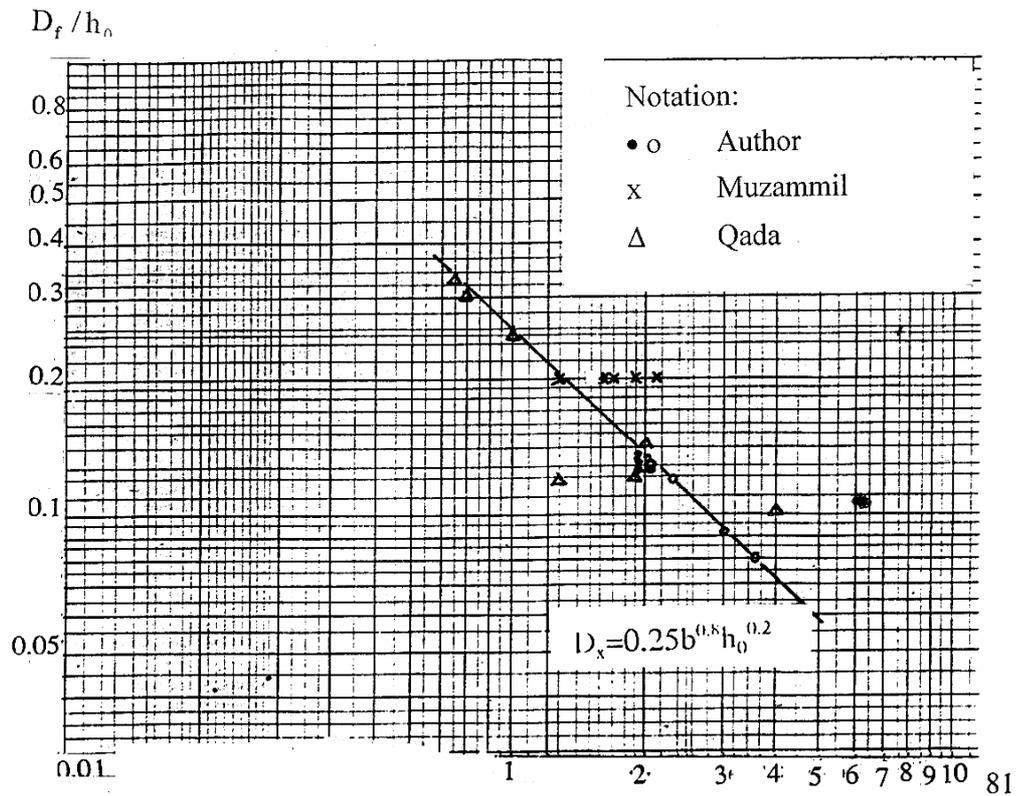
Fig.7. Variation of  $(\frac{D_f}{h_0})$  with  $(\frac{b}{h_0})$  in uniform flow
