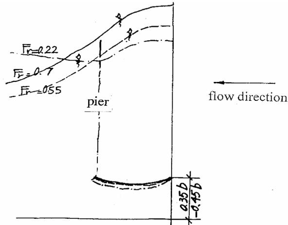
Fig.2. Vertical separation line and vortex zone on the pier side surface.
